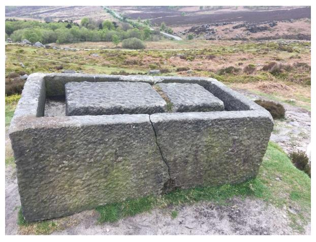
A disaster for the mason, this block had been moved and fell apart under its' own weight as the inside was being chiselled out.
