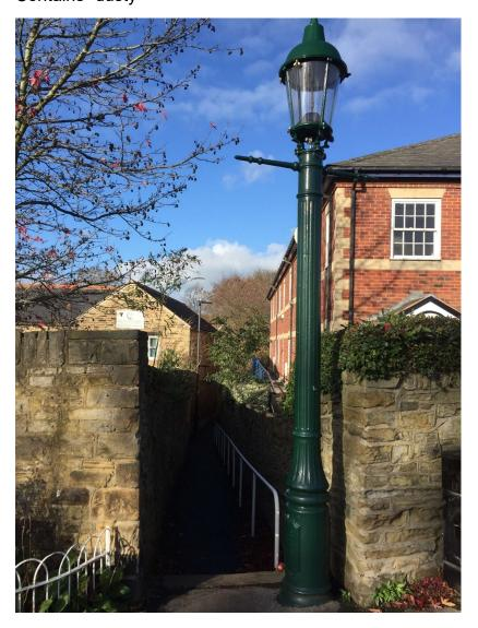
One of several 'Sewer Gas Destructor' lamps from 1890. This one is Grade II listed by English Heritage. The sewer gas collects at the high point of sewer pipes and to avoid possible explosions, is tapped into this patented lamp where is is mixed with town gas and burnt by a very hot flame which destroys the smell. Sheffield, being hilly, needed 84 of these. There is another nearby on Brincliffe Edge Road.
