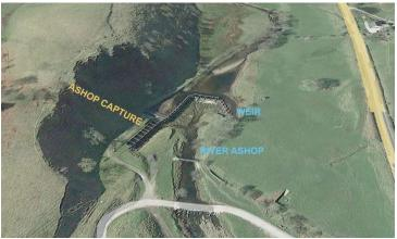
Just before the River Ashop is jointed by the River Alport a clever capture takes place. The River Alport water escapes left through a weir and the captured water is led right into a short tunnel.
